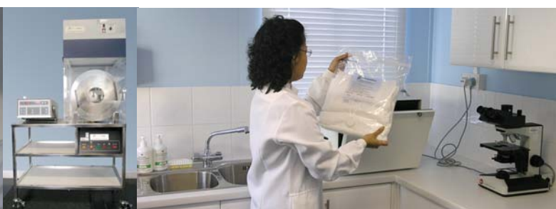
Testing for particulate cleanliness of processed wipes is performed at Micronclean using the Helmke drum method
